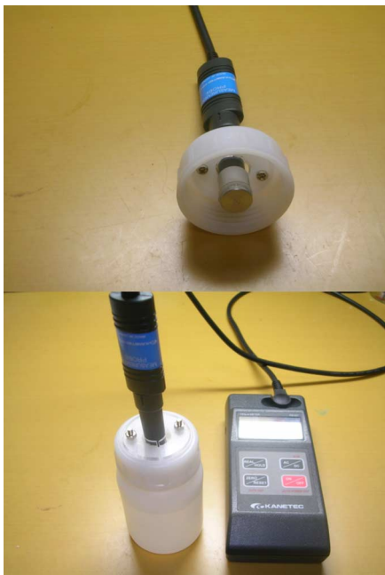
Fig. 2. Set up of sample-tube and Tesla-meter (lower) and hole sensor held with a cap (upper).
